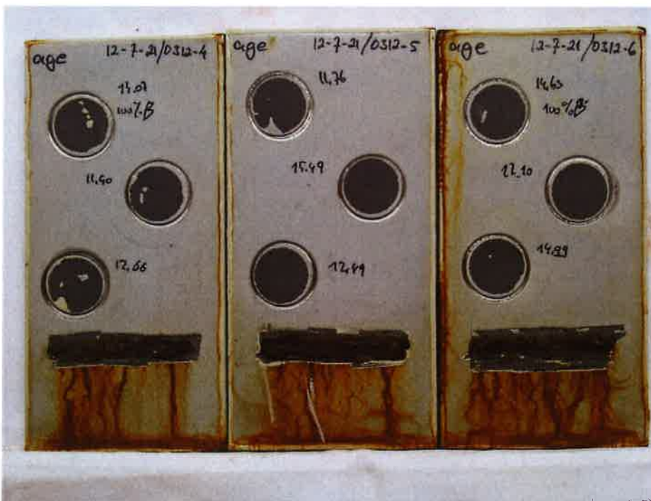
Photo 2: Panels 4, 5 and 6 after 1680 hours Cyclic Ageing test
